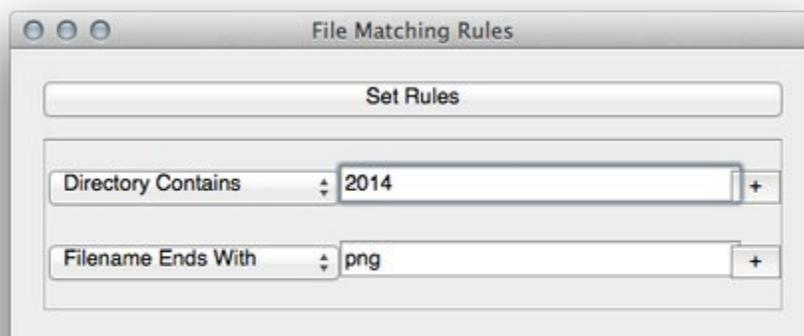
4. Often, it is helpful to save a rules set and scan rules to reuse—for example, if a complex rules set is highly detailed, or in order to create a toolbox of rules sets to use for different formats. Under File -> Save Template, templates can be saved for later use; they are loaded again via File -> Load Template.
